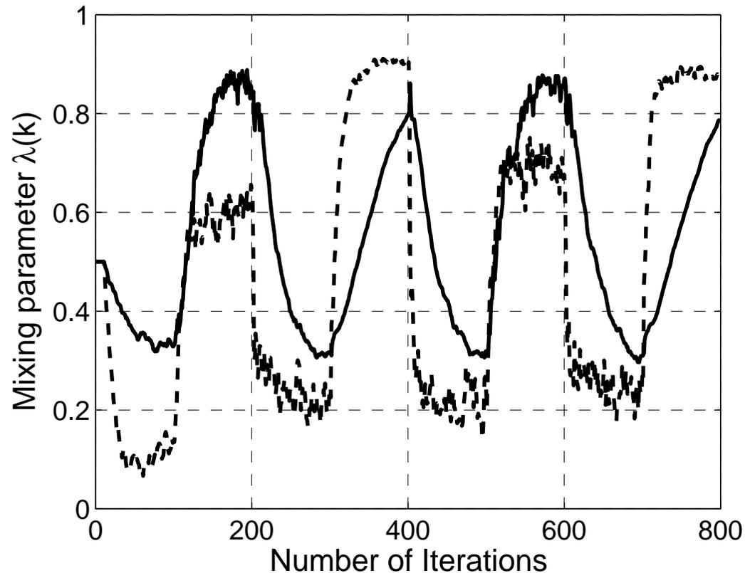
⇒ output of the convex combination is dominated by the filter most appropriate for the input signal characteristics
